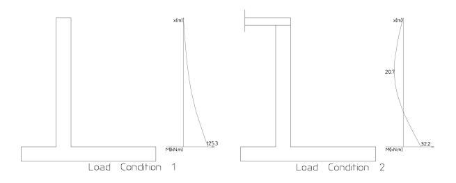
Positive Moment in Front-face of Stem: Load combination two is critical
